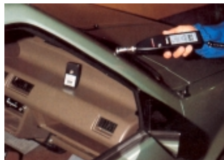
Control of tightness with ultrasonic transmitter
