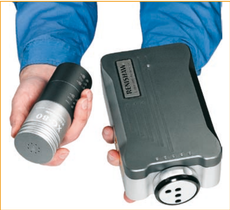
XL-80 laser (with optional universal shutter) and XC-80 compensator
