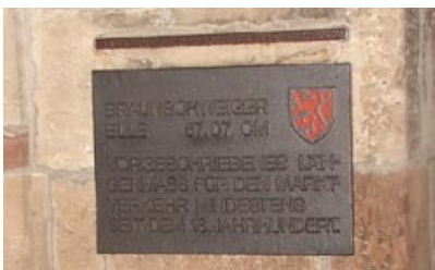
In the Town Hall in Braunschweig, Germany, there is a length of steel mounted on the wall. In the 1700s, this type of bar served as a very public dimensional standard for the cloth merchants in town. Source: Mahr Federal Inc.
