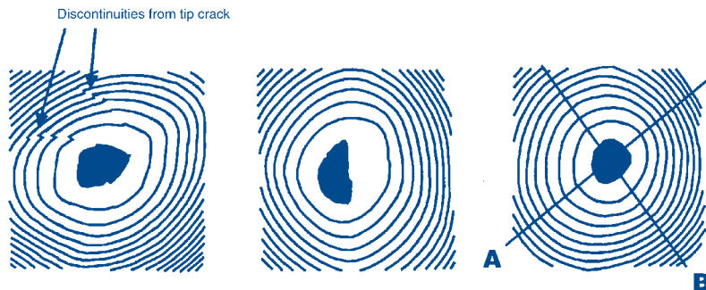
These are examples of skeletonized microinterferograms of diamond stylus tips showing surface discontinuities. The micrograph is a “contour map” of the tip so that all points on a given ring are equidistant from the reference optical flat. Source: Mahr Federal Inc.
