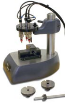
Because of tightening tolerances it became impossible to do parallelism checks with off-the-shelf gaging to meet the 0.0001-inch requirement for this application. But by combining standard components with modified components and electronic signal conditioning, the parallelism can now be checked right at the point of manufacture by the machine operators. Source: Mahr Federal Inc.
