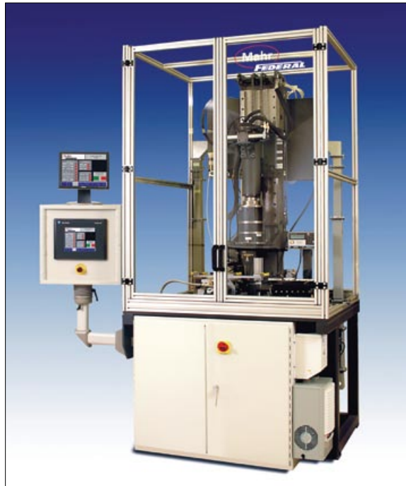
This fully automatic gage does 100% inspection of 21 characteristics on thousands of cylinder liners, in 12 seconds each. Results are recorded, classified and marked, and information about the process is fed back to the machine tool for offset compensation. No set of manual gages nor any number of inspectors were capable of the throughput this operation required. Source: Mahr Federal Inc.
