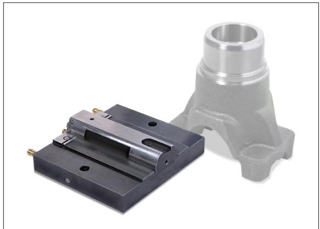
It would be nice if all measurements were simple IDs or ODs, but they are not. Here the air gage creates a matching part and the air jets are not on the diameter but on the chord. Source: Mahr Federal Inc.
