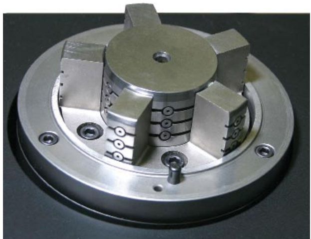
Electric motor stators offer a unique measurement challenge. In this example, 24 separate air jets combine to provide all the dimensional and form information from a single bench gaging station. Source: Mahr Federal Inc.
