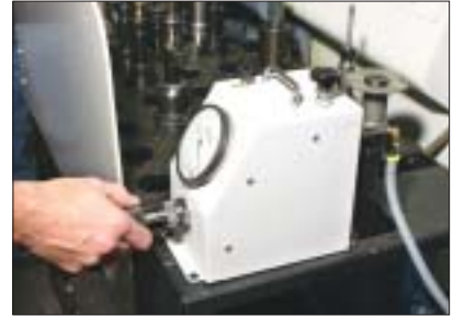
Air gaging has increased in popularity in recent years as part tolerances have gotten tighter. It is readily used in production environments and the gages even help clean parts by blowing dirt away. Source: Mahr Federal Inc.
