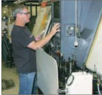
Air gaging is ideal for part inspection at the machine because it is fast and easy to use. Source: Mahr Federal Inc.
