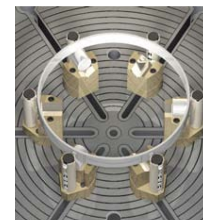
Inside and outside diameter measurements are possible by rotating the gageheads
