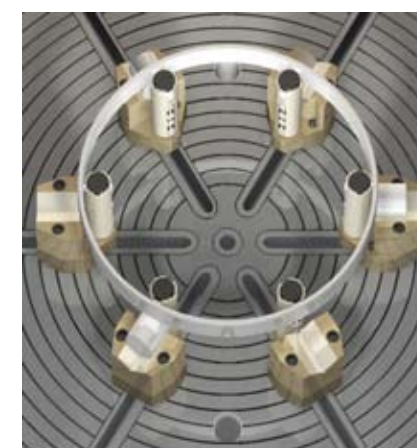
Inside and outside diameter measurements are possible by rotating the gageheads
