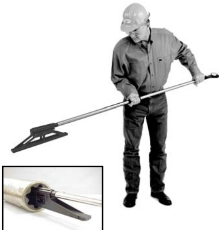
Inspects Internal Diameters of Stators
